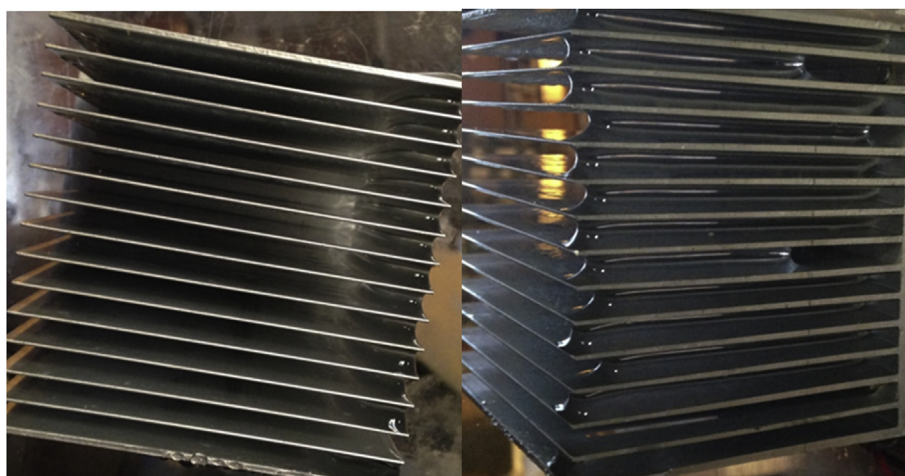
Fig. 13. Rotated heatsink at 75° angle.
