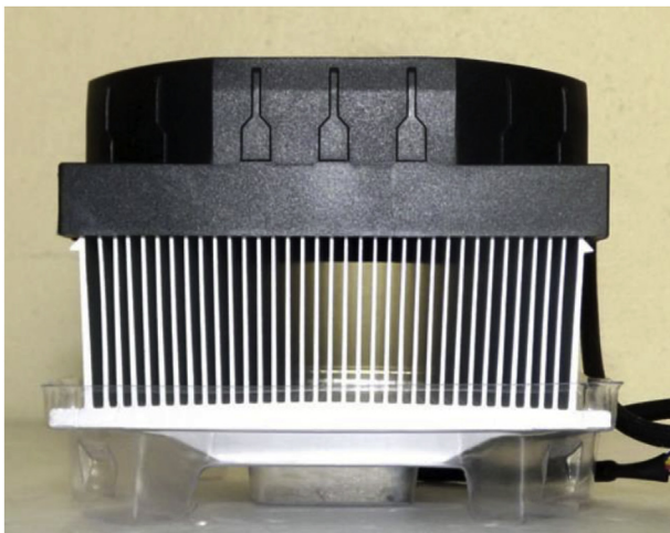
Fig. 1. Heatsink and fan combination used for the heat rejecting side of Peltier element—hot side heatsink.
