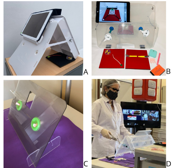
Fig. 1. Training Box Assembly (A) 3D-printing adapted training box with smart device as a functional camera and screen. (B) Low cost endotrainer with smart device as a functional camera and screen. (C) Other option of 3D-printing endotrainer. (D) Workstation Assembly. A second device is used as an external camera for assessing ergonomics.
