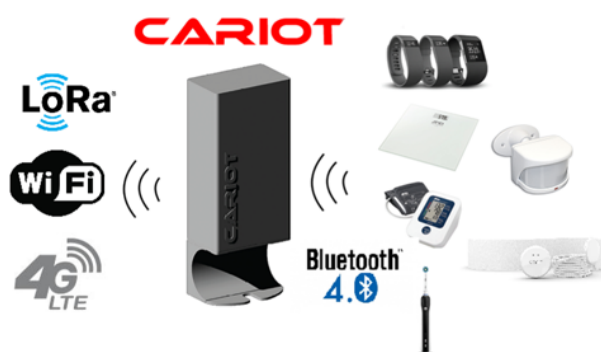
Figure 1: The CARIOT homecare sensing platform (center of the image) communicates with an Oral-B electrical toothbrush and sends the data via a range of different communication protocol standards, Lora, WiFi or 4G to the automatic adherence aid system.
