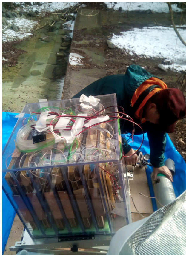
Figure 3. A photograph about the installation of muographic observations system at one of the sabo dams of Karasu River
