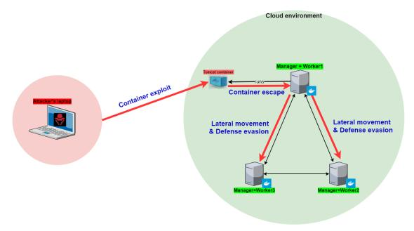
Figure 4. Diagram of the attack steps.
