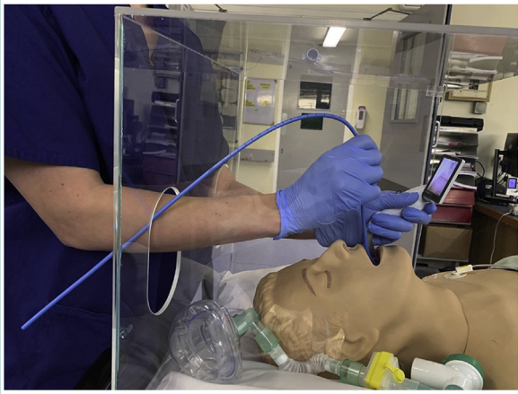
Fig 4 Usability testing of a novel 'intubation box' for simulated tracheal intubation using a McGrath™ MAC videolaryngoscope (Medtronic, Minneapolis, MN, USA) and a gum-elastic bougie. 15 Reproduced with permission.
