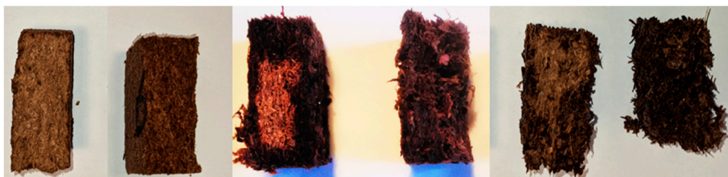
Figure 2. Water penetration over the cross section of the tested sample: fibre length 1.6 mm, wet and dry (left); fibre length 4 mm, wet and dry (middle); and fibre length 7 mm, wet and dry (right).
