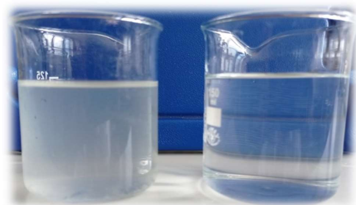
Figure 4. Wastewater before (a left side) and after (a right site) the microfiltration process on TAMI membrane with pore size of 0.45 mm.
