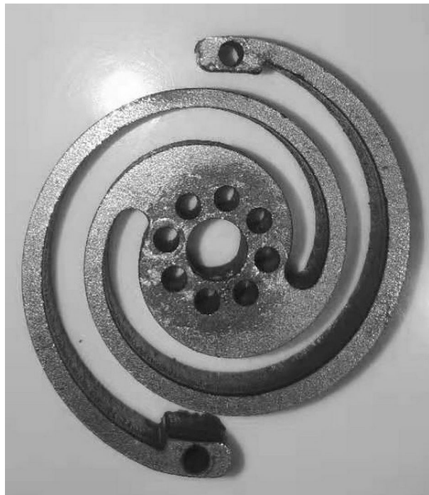
Figure 9. Manufactured planar spiral spring.
