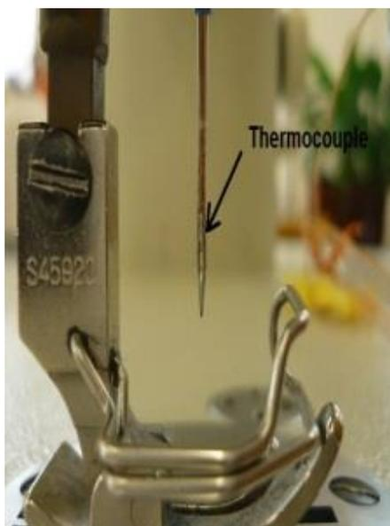
**Figure 2.** Thermocouple embedded in the needle.
