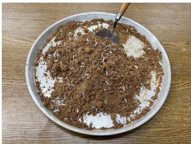
Figure 6. Sand mixed with a 15 mm fiber content of 0.2%.
