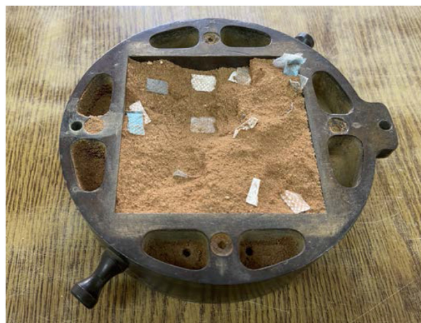
Figure 12. Sheared sample reinforced with mask chips.
