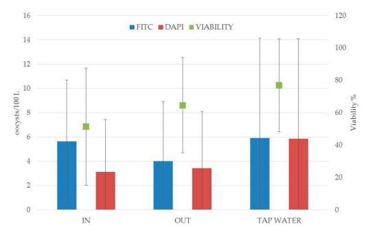
**Figure 1.** Mean and standard deviation (SD) of the concentration of *Cryptosporidium* spp. and number of oocysts viable at the different sampling points. The percentage of viable oocysts in the sample was calculated using DAPI staining.
