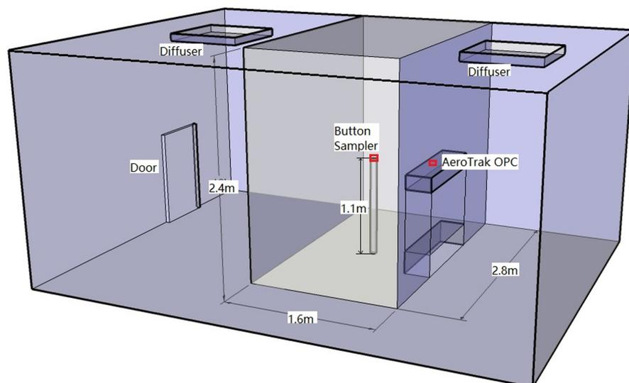
**FIGURE 1** Design of the test chamber (the structure in the middle of a room with dimensions of 2.8 m length  $\times$  1.6 m width  $\times$  2.4 m height) and placement of equipment used in resuspension experiments.
