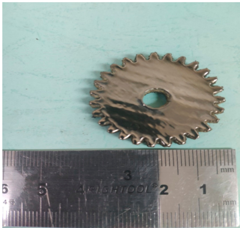
Figure 8. SLM-fabricated Zr_{60}Fe_{10}Cu_{20}Al_{10} BMG part (diameter 35 mm and height 5 mm).
