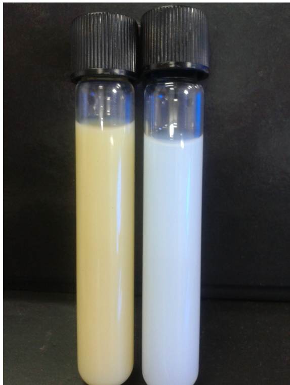
Figure 2 Nanoemulsions obtained by low energy method. HFNE shown in left side and blank nanoemulsion shown in right side of the picture.
