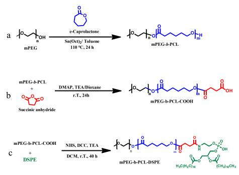
**Scheme 1.** CL polymerisation starting from mPEG as an initiator via ROP (**a**), reaction of PEG-*b*-PCL with succinic anhydride (**b**) and conjugation of carboxylated copolymers with DSPE through amidation (**c**).
