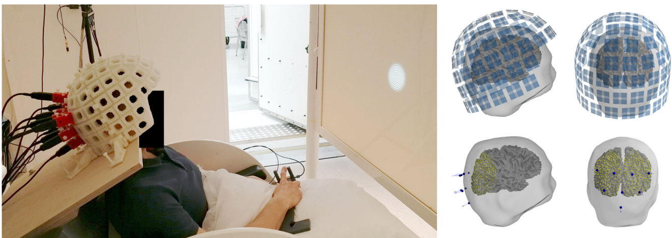
FIGURE 1 Left: The optically pumped magnetometer (OPM) measurement setup in the magnetically shielded room (MSR). Right: SQUID (top) and OPM (bottom) sensor positions with respect to the head of a representative subject. The source space used for OPM source estimation is shown as yellow points
