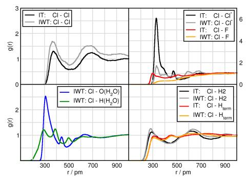
Figure 5. RDFs between the Cl(TiCl<sub>4</sub>) and all compounds in systems IT and IWT.
