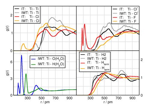
**Figure 4.** RDFs between the  $Ti(TiCl_4)$  and atoms of the different compounds in systems IT and IWT. Please note the y-axis have different scales and that Cl marks the chlorine atom from  $TiCl_4$ , while  $Cl^-$  stands for the chloride anion.
