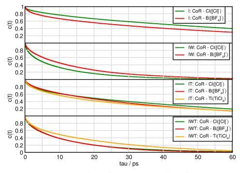
**Figure 9.** Continuous autocorrelation of aggregates associated with the cation. Aggregates were determined at approximately their first minimum in the RDF.
