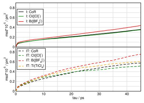
Figure 7. Mean square displacement of particles in systems I and IT.
