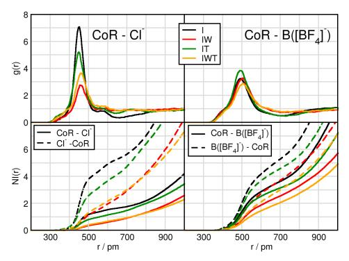
**Figure 1.** Radial distribution functions (RDFs) and number integrals (NIs) between the center of imidazolium ring CoR and chloride  $Cl^-$  (left panels), and the boron atom of tetrafluoroborate B([BF<sub>4</sub>]<sup>-</sup>) (right panels) in systems I (black), IW (red), IT (green) and IWT (orange).
