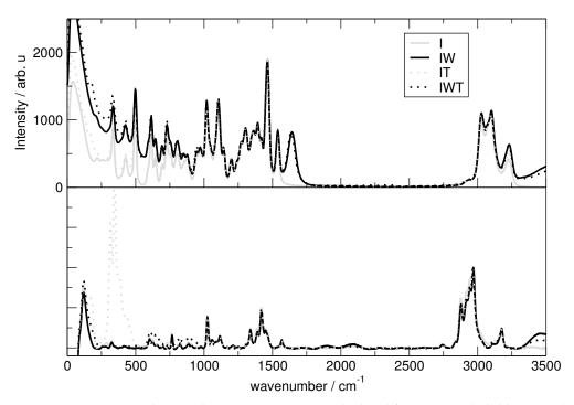
**Figure 12.** Upper panel: Complete power spectrum calculated for system I (solid line, gray), IW (solid line, black), IT (dotted line, gray) and IWT (dotted line, black) Lower panel: Experimental Raman spectrum with the same mixing ratio as theoretical systems.
