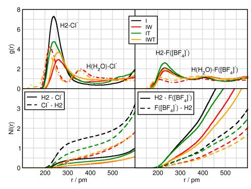
**Figure 2.** RDFs and NIs between H2 of the cation (solid) or H of  $H_2O$  (dashed-dotted) and the contact atoms of the anion  $Cl^-$  (**left panels**) and the fluorine atoms of tetrafluoroborate  $F([BF_4]^-)$  (**right panels**) in systems I (black), IW (red), IT (green) and IWT (orange).
