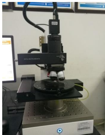
Figure 8. Three-dimensional topographic imager (Zeta-20).
