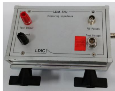
Figure 6. Quadropole for PD measurement according to the standard IEC 60270.
