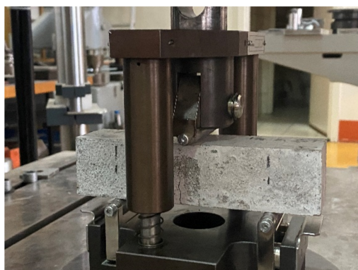
Figure 2. Toughness testing; positioning of the specimens and testing frame.
