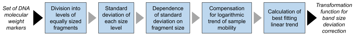
Fig. 2. The principle of the derivation of the transformation function for eliminating the trends in band size deviation.
