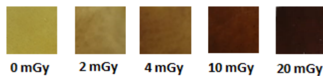
Figure 2. Direct perceived color change of PVA/Ag + /NBT films irradiated with different X-ray doses.
