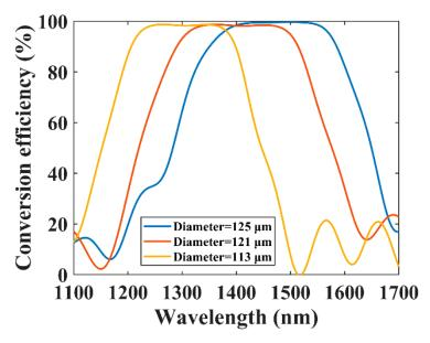
**Figure 6.** The conversion efficiency of three BLPFGs with a diameter of 113  $\mu$ m, 121  $\mu$ m, and 125  $\mu$ m, respectively.
