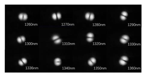
Figure 7. The output modes of the BLPFG in its working window.
