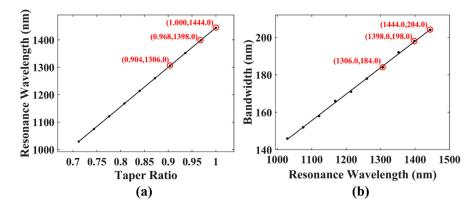
**Figure 3.** (**a**) The change in the dispersion turning point with the taper ratio. (**b**) The change in the 15 dB bandwidth with the dispersion turning point.
