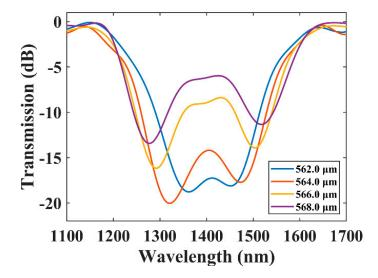
**Figure 5.** The transmission spectra of BLPFGs. The cladding diameter is 121  $\mu$ m, and the periods are 568.0  $\mu$ m, 566.0  $\mu$ m, 564.0  $\mu$ m, and 562.0  $\mu$ m.
