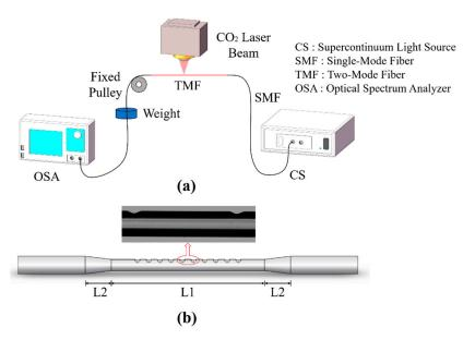
**Figure 4.** (a) Schematic diagram of the BLPFG preparation. (b) Schematic diagram of the BLPFG and micrograph of one period in the taper waist.
