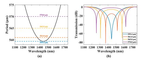
**Figure 2.** (a) The LPFG period versus the wavelength variation curve. (b) The LPFG transmission spectra with different periods.
