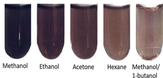
Figure 1. Degree of turbidity on the reaction of mixture solvent-lycopene and DPPH radicals.
