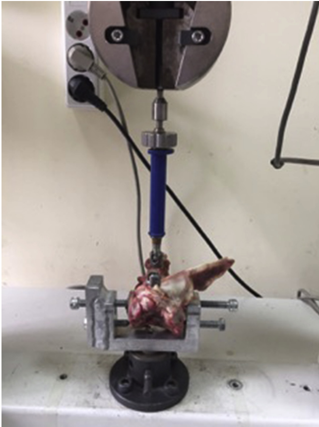
Fig. 2. The pedicle screw pull-out strength was tested using the a 10 kN capable Shimadzu (Shimadzu Corp., Kyoto, Japan) Autograph AGS-J model universal testing machine at a rate of 5 mm/min.
