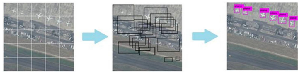
Figure 5. YOLO model divides image into S \times S grid and calculates confidence scores with B bounding boxes and predictions are enclosed into (S \times S) \times (B * 5 + C) tensor.
