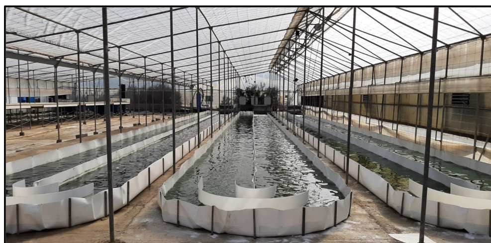
Figure 1. Pilot-scale raceway reactors located inside a greenhouse in Almería, Spain.
