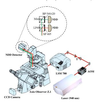
**Figure 1. Experimental setup of a nonlinear optical microscopic system.** CCD: charge-coupled device, AOM: acoustic-optic modulator, T<sub>1</sub>: telescope, SP: short-pass filter, BP: band-pass filter, LP: long-pass filter, NDD: Non Descanned Detector. The SHG (red lines) and TPEF (green lines) are collected in a transmitted light configuration. doi:10.1371/journal.pone.0069186.g001
