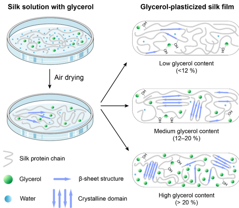
Figure 6. A schematic illustration of the role of glycerol in plasticizing silk proteins during the film fabrication.
