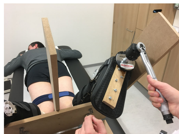
Fig. 3 Internal rotation with 6 Nm torque
