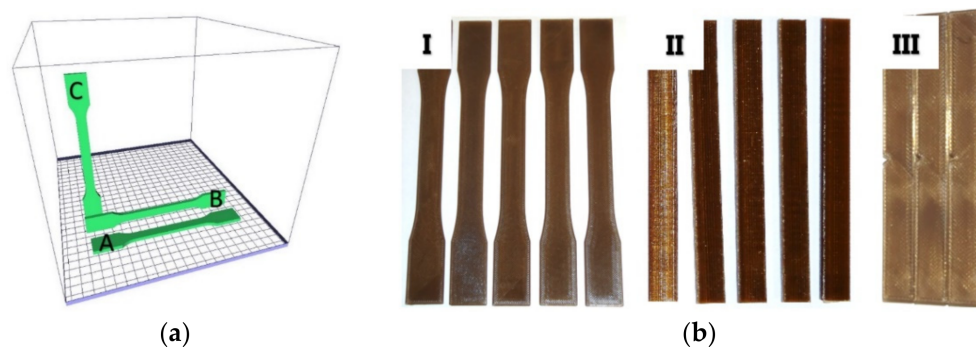
Figure 1. (a) Geometric orientation of the printed samples with the marked printing directions: (A) through thickness, (B) transverse, (C) longitudinal; (b) printed specimens used for: I—tensile testing, II—three-point bending testing, III—impact testing.
