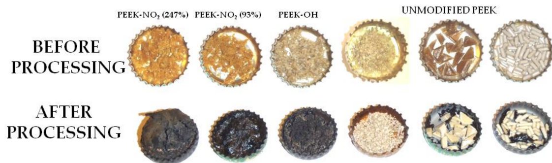
Figure 11. Results of thermal treatment of the obtained PEEK modification products.
