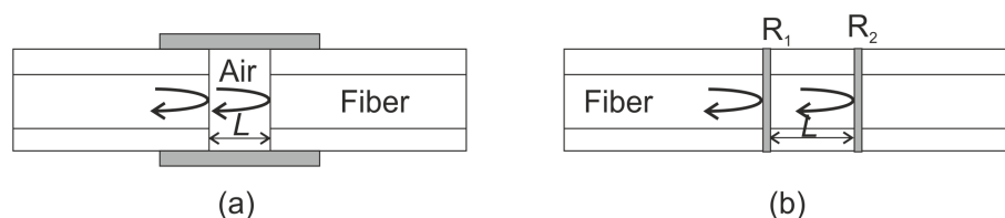
Figure 4. Principle of FPI (a) extrinsic (b) intrinsic (based on reference [47]).
