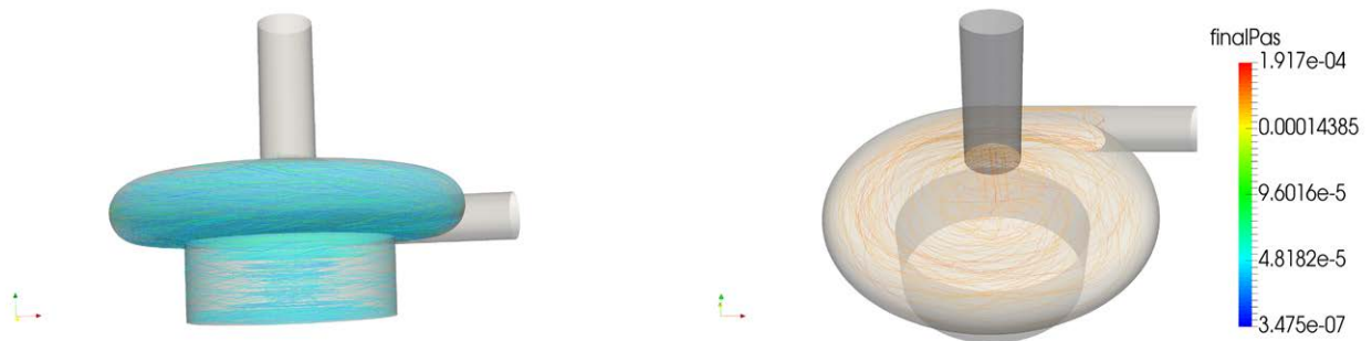
Figure 4. Path-lines for the CentriMag, adult mode of most activated platelets (left) and longest residing particles.
