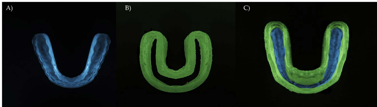
Figure 1. Hybrid occlusal splint mouthguard design (Kalman et al., 2022 [5]). (A) Polycarbonate as a rigid inner portion, (B) ethylene vinyl acetate used in the axial flexible flanges, and (C) the final modulated appliance assembled as the novel HMG.
