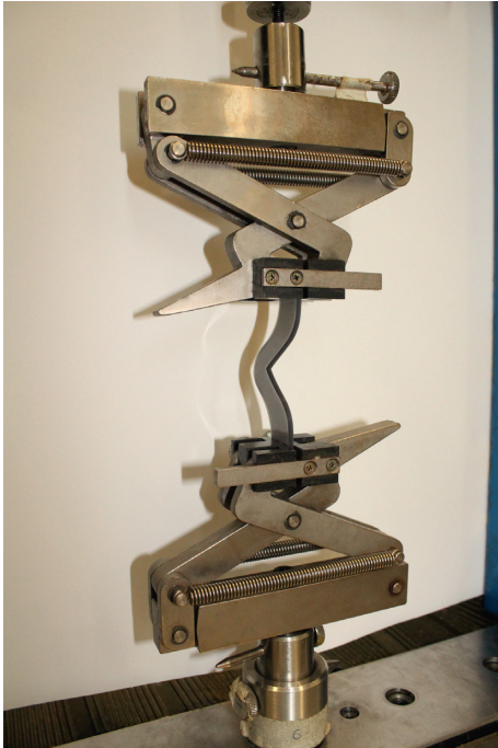
FIGURE 3: Specimen positioned for tear test.
