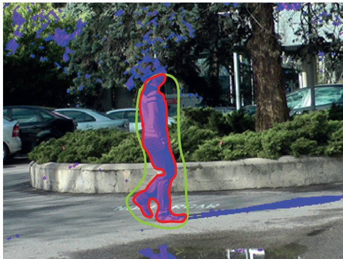
Figure 8. Example of using the intelligent mode combined with the motion detection tool. The difference mask is shown in semitransparent purple. The contour drawn by the user with the intelligent mode is shown in red. The contour resultant from the combination of the motion mask and the contour manually drawn is shown in red.
