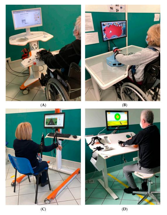
**Figure 1.** Robotic and sensor-based devices used to treat the upper limb: (**A**) Amadeo (Tyromotion); (**B**) Motore (Humanware); (**C**) Diego (Tyromotion); and (**D**) Pablo (Tyromotion).
