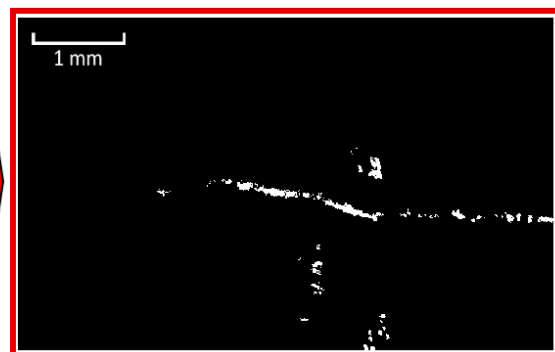
Slice from the Binary Crack and Void Image
