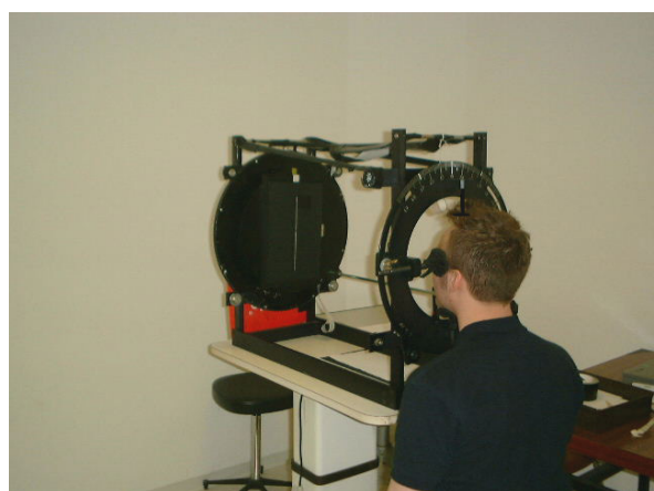
Figure 1 The experimental apparatus. During the experiment, the whole apparatus was covered by a black cloth (to prevent contextual visual cues).
