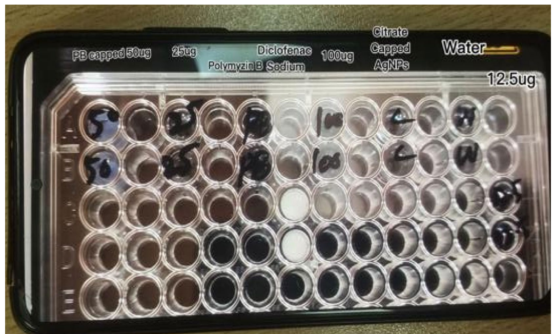
Fig. 10. Egg albumin combinations made on 96 well plates for Elisa reading.
