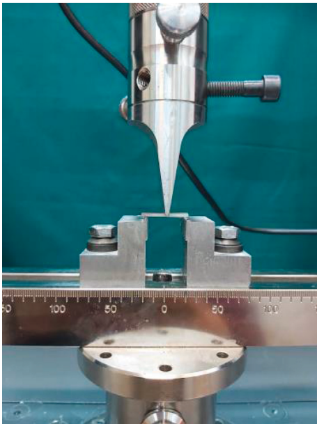
FIGURE 2: Testing the flexural strength through three-point bend test.
