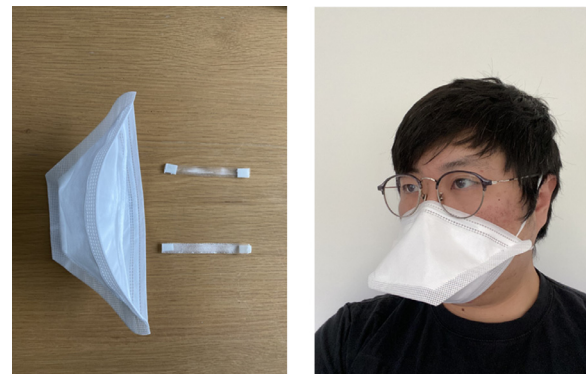
Fig. 1. Photograph of duckbilled-mask used, and sampling strips that are fixed within the inside of the mask, that can be removed for analysis.
