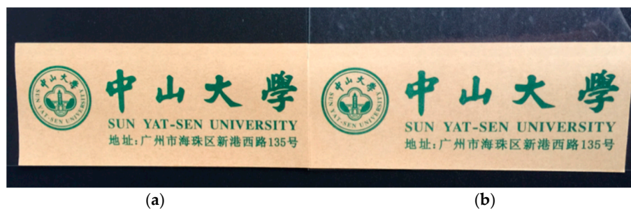
Figure 15. Photographs of (a) bare PET film and (b) PET-(QL) 19 composite film in front of a printing paper.
