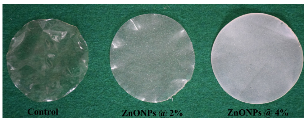
Fig. 3. Photographs of the ZnONP-agar nanocomposite films.
