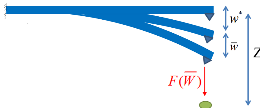
Figure 1. The displacements of the tip in static equilibrium state and vibration state.
