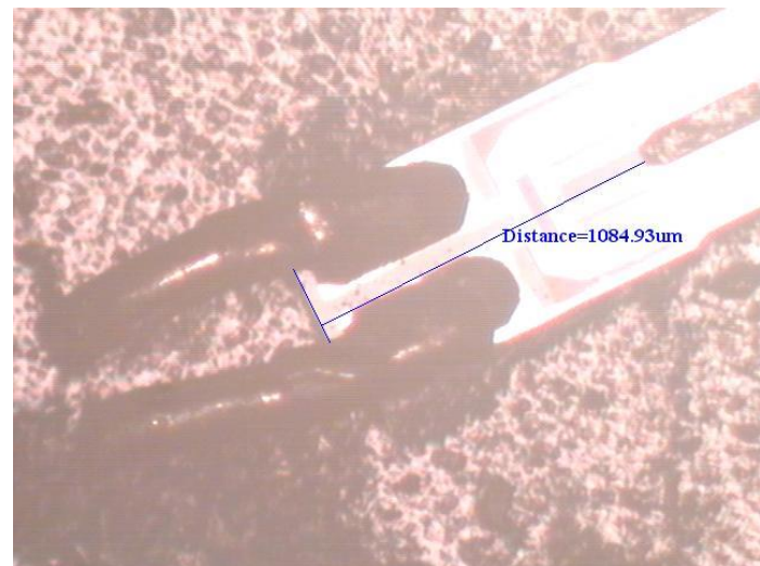
Figure 16. Determination of the length of the proof mass from a microscope image.
