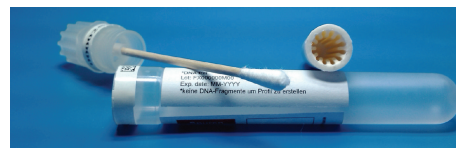
FIGURE 1: forensiX evidence collection tube, disassembled, with cotton swab and the SafeDry desiccant insert with a serrated inner surface.
