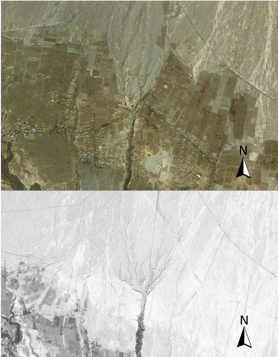
Fig. 8 Comparison of a modern view of the landscape north of Murtuq in Turpan on the Corona KH-4B satellite imagery (under) and the Esri Satellite basemap (above). Several karez lines, roughly running north-south are visible and the destruction by the agricultural expansion is evident (USGS Corona Imagery, Esri Basemap)
