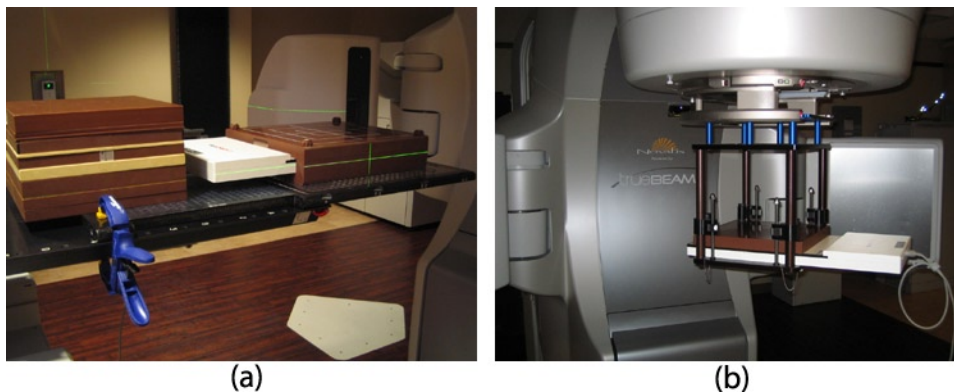
FIG. 1. MapCHECK 2 device set up for measuring IMRT validation plans: (a) MapPHAN QA using MapPHAN-MC2 on an extended tennis-racket-type grid couch top, and (b) IMF QA using the isocentric mounting fixture (IMF).
