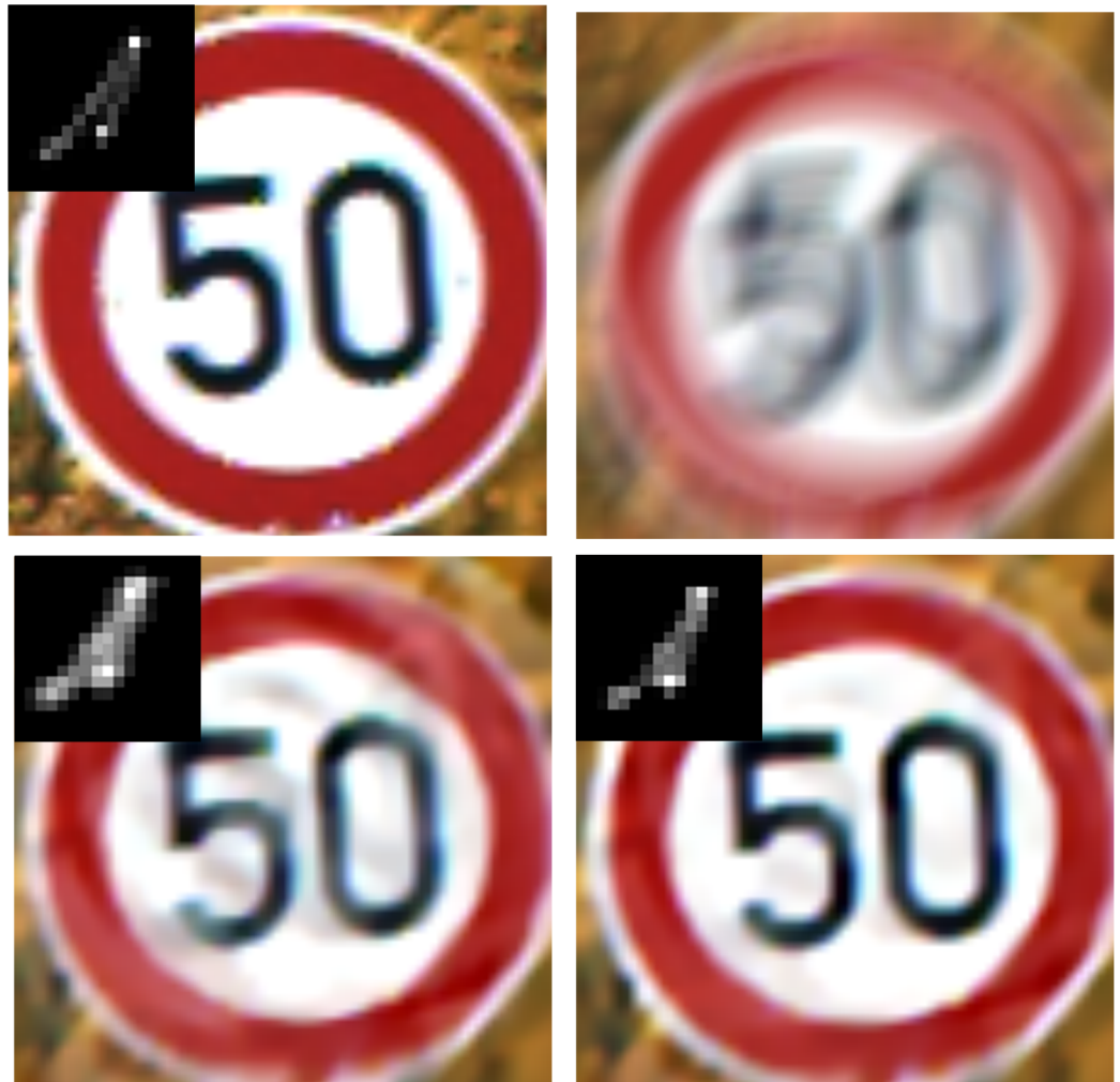
Fig 10. Deblurring results for synthetic traffic signs during sunny day time. (a) denotes the input image and real blur kernel. (b) denotes the blurred image. (c) and (d) denote the deblurring results of Pan[9] and our method, respectively.
