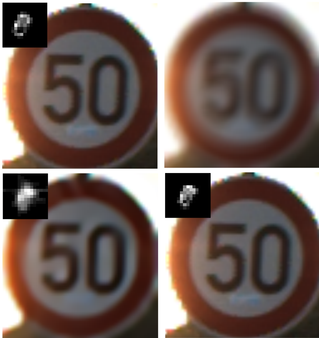
Fig 13. Deblurring results for synthetic traffic signs during late morning. (a) denotes the input image and real blur kernel. (b) denotes the blurred image. (c) and (d) denote the deblurring results of Pan[9] and our method, respectively.
