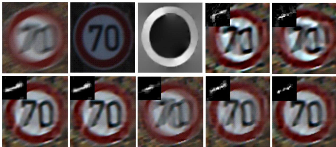
Fig 9. Example of real captured image. (a) denotes the real captured image. (b) denotes the matched exemplar. (c) denotes the predicted \nabla S . (d)–(j) denote the deblurring results of Krishnan[12], Xu et al.[17], Shan[15], Xu & Jia[7], Levin[16], Pan[9] and our method, respectively. In (d)–(j), each image includes deblurring image and estimated kernel.
