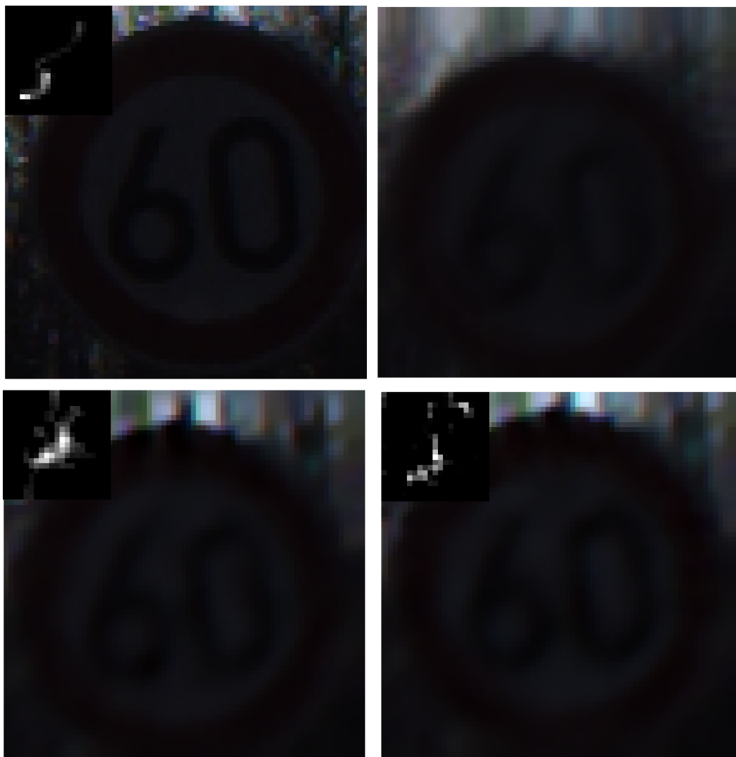
Fig 14. Deblurring results for synthetic traffic signs during early evening. (a) denotes the input image and real blur kernel. (b) denotes the blurred image. (c) and (d) denote the deblurring results of Pan[9] and our method, respectively.
