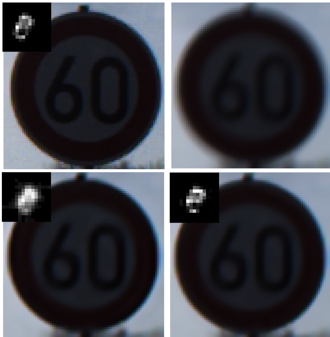
Fig 11. Deblurring results for synthetic traffic signs during cloudy day time. (a) denotes the input image and real blur kernel l . (b) denotes the blurred image. (c) and (d) denote the deblurring results of Pan[9] and our method, respectively.
