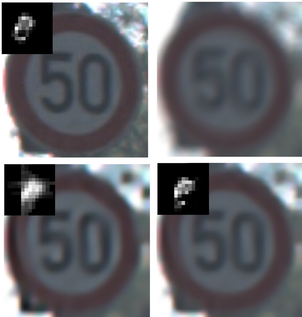
Fig 12. Deblurring results for synthetic traffic signs during foggy day time. (a) denotes the input image and real blur kernel. (b) denotes the blurred image. (c) and (d) denote the deblurring results of Pan[9] and our method, respectively.
