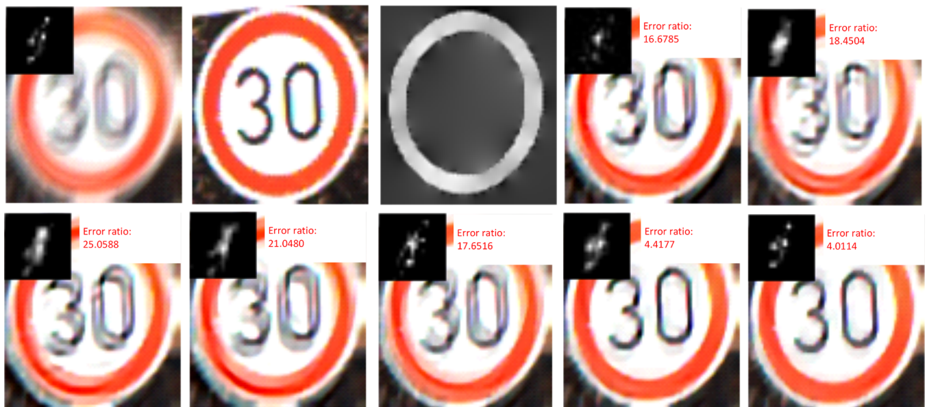
Fig 7. Image deblurring comparison for synthetic images. (a) denotes the input image and real blur kernel. (b) denotes the matched exemplar. (c) denotes the predicted \nabla S . (d)–(j) denote the deblurring results of Krishnan[12], Xu et al.[17], Shan[15], Xu & Jia[7], Levin[16], Pan[9] and our method, respectively. In (d)–(j), each image includes deblurring image, estimated kernel and error ratio.
